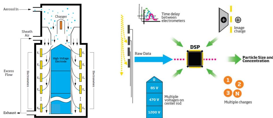
Fig. 1: Schematic diagram and data inversion of the EEPS.
