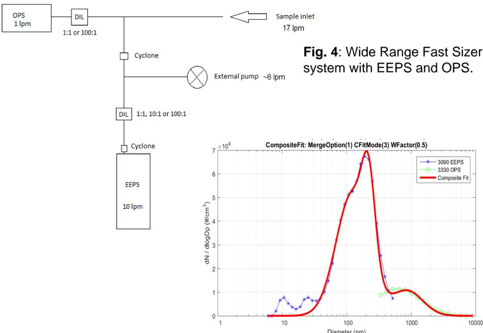
Fig. 4: Wide Range Fast Sizer system with EEPS and OPS.
