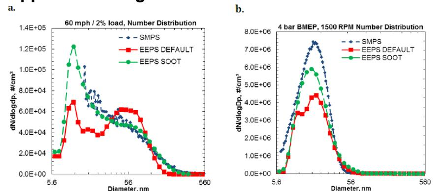
Fig.3: Default and Soot matrices compared to SMPS for a GDI vehicle (a) and light duty diesel engine (b)
