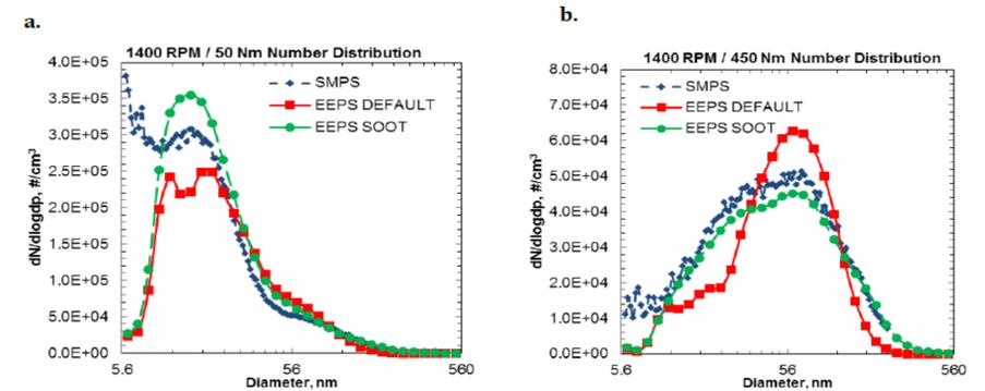
Fig. 2: Default and Soot matrices compared to SMPS for HD diesel engine running at 1400 RPM, 50 Nm (a) and 450 Nm (b)
