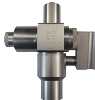
PM2.5 Very Sharp Cut Cyclone (VSCC) 16.67 LPM
