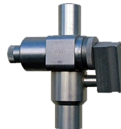
PM2.5 Sharp Cut Cyclone (SCC) 16.67 LPM
