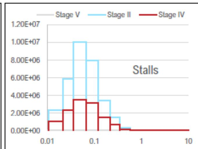
Number size distributions of STAGE IV, V, and II during different drive cycle phases (1/cm<sup>3</sup>). Stage V is almost invisible due to substantially lower concentration levels (3 orders of magnitude). Note that the Y-axis scale is different between the graphs.
