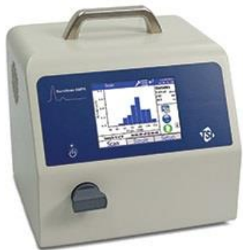
Nanoscan SMPS 3910 粒径範囲10 nm~420 nm
