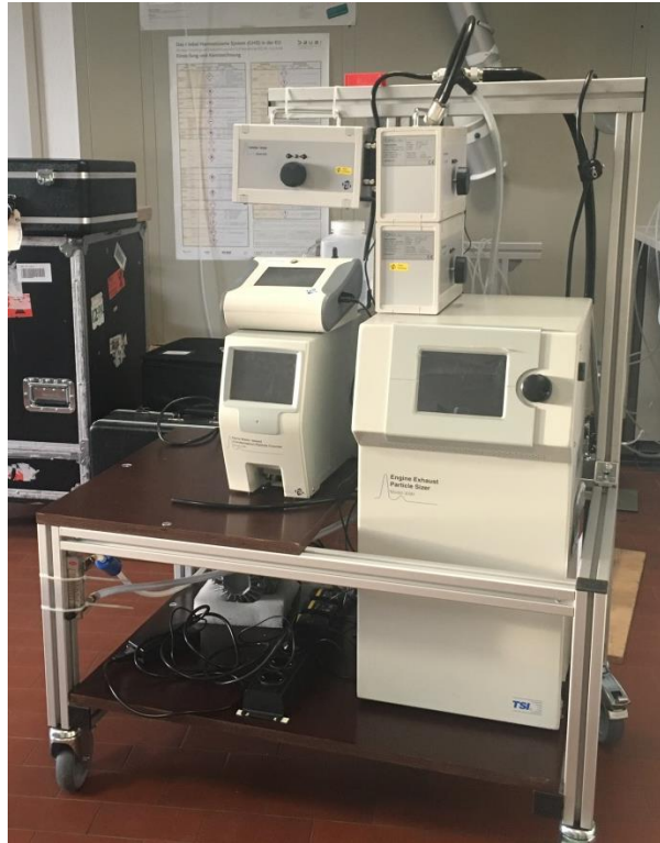
Figure 2: Photo of the wide range fast sizer system with EEPS spectrometer and OPS as it was used for the brake wear emissions measurements. In addition to the optional three diluters pictured, a Nano water-based Condensation Particle Counter (N-WCPC) is included as a reference for total particle concentration.
