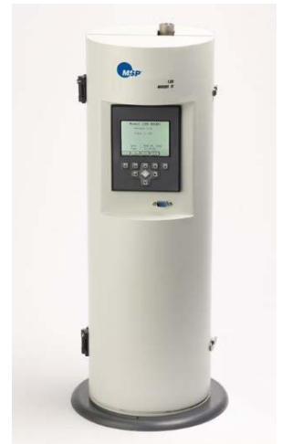
Model 125R 10 L/min 13 Stage MOUDI II impactor
