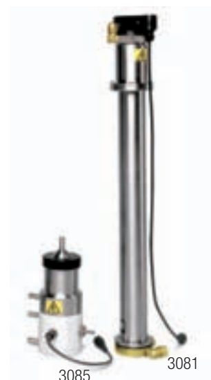
DMA's contain highly polished surfaces for high-resolution particle size classification (above). The Series 3080 offers a choice of two DMA's (right).
