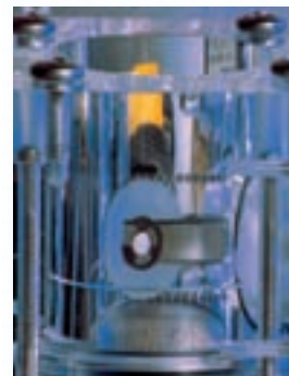
A bed of bronze beads inside the Model 3400A breaks up powder agglomerates before dispersion.
